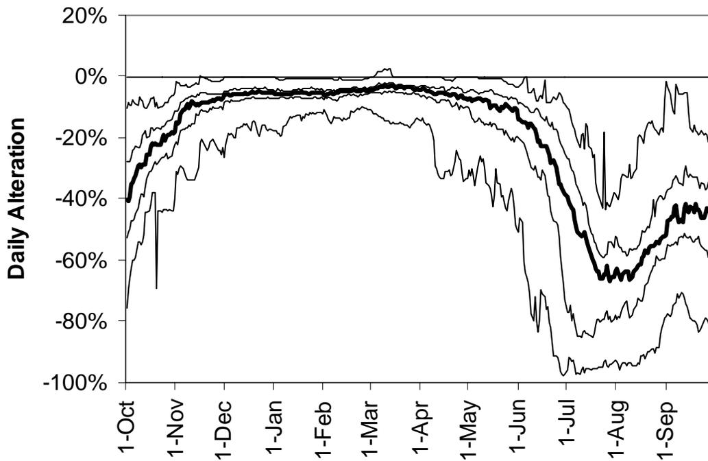
FIGURE 32.—Median, 25<sup>th</sup> and 75<sup>th</sup> percentiles, and extremes of daily flow alteration in Fall River at Chester for water years 1972-2002.
