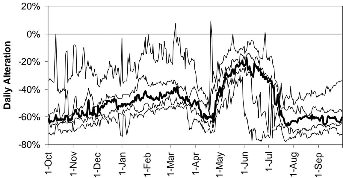
FIGURE 26.—Median, 25<sup>th</sup> and 75<sup>th</sup> percentiles, and extremes of daily flow alteration in Fall River at Squirrel 22 August 1993 to 30 September 2002 (post power plant).
