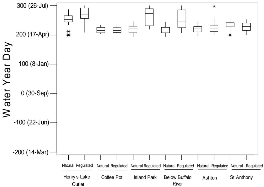
FIGURE 44.—Date of maximum flow for natural and regulated hydrologic regimes on the Henry's Fork.
