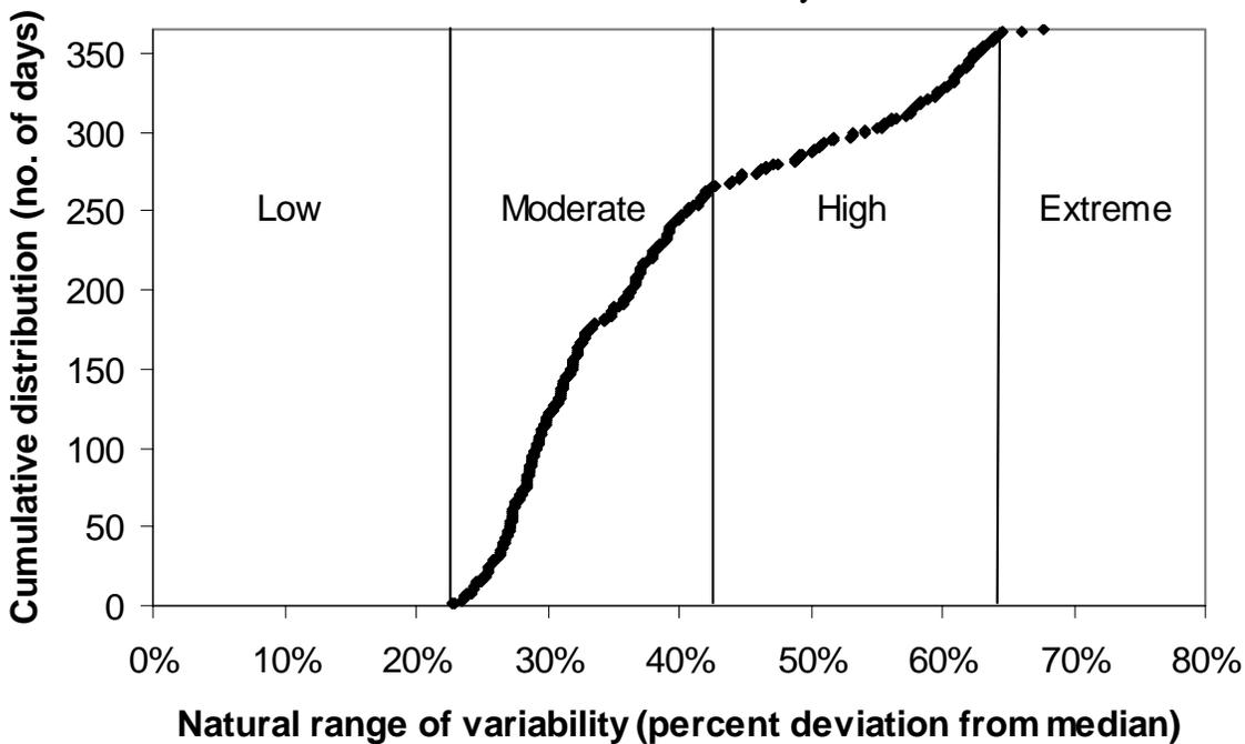
b. Cumulative frequency distribution and corresponding definitions of hydrologic alteration.
