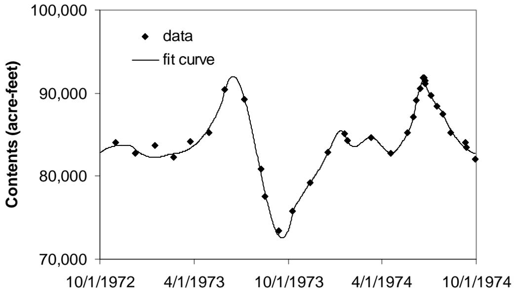
FIGURE 2.—Example of Henry's Lake contents curve fit to data collected prior to installation of the continuous recording gage using a combination of polynomial regression and splines.
