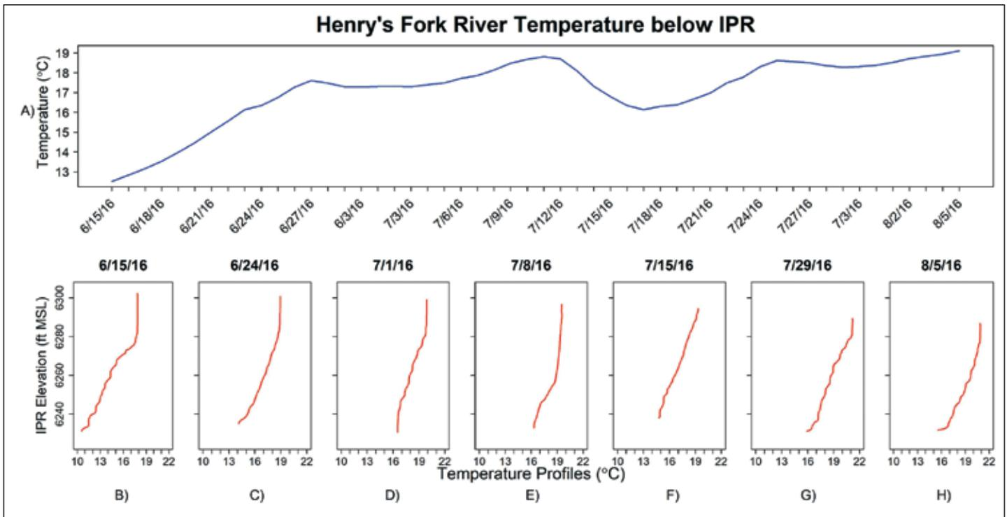
Figure 5. 5A shows water temperature ( $^{\circ}\text{C}$ ) trends collected in the Henry's Fork River from June 15 to August 5, 2016. 5B-H show water temperature profiles collected at IPR Gates. Note in figures 5B-H the top of each profile starts at a lower elevation as the summer progresses, reflecting reservoir draft
