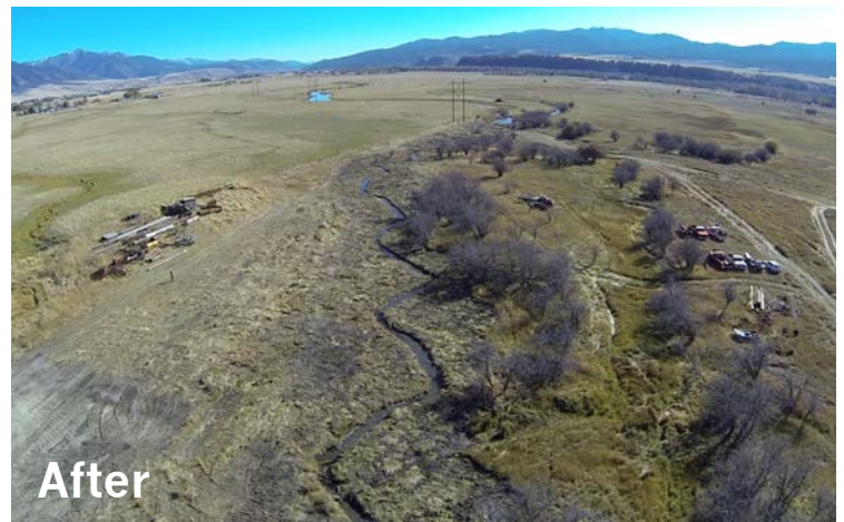
Restoration work increased sinuosity in the creek, made the channel more narrow, and increased water velocity, resulting in cooler water temperatures and improved trout habitat.
