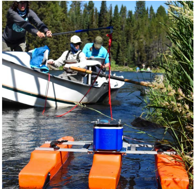
Christina and HFF staff measure streamflow using an Acoustic Doppler Current Profiler (ADCP) unit provided by Fremont-Madison Irrigation District (FMID) as part of ongoing partnership. Thank you FMID!
