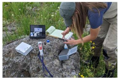
The research also involves nutrient analysis, assessment of total Nitrogen and Phosphorus levels, turbidity samples, water temperature and pH. In this photo, HFF staff member Kamberlee Allison is conducting a titration to test the alkalinity of the water sample.
