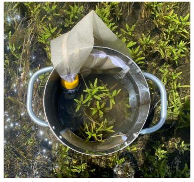
Sampling locations are selected randomly as GPS points, the sampler is set down in the river channel and macrophytes within the sampler are collected. Then they are identified by species, taken to the lab, dried, and measured to attain biomass (total mass of organisms in a given area or volume).
