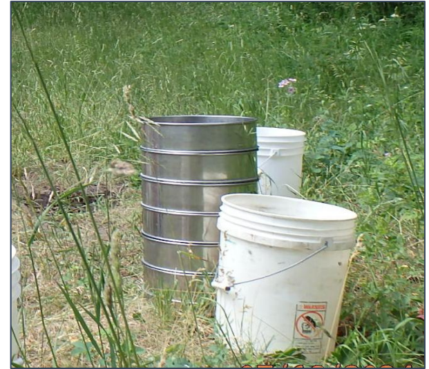
Separate sediment sizes by volumes and calculate total percentages.
