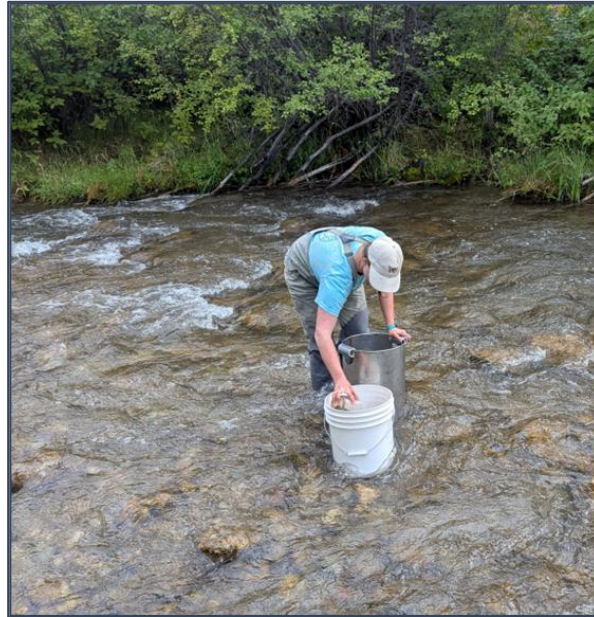
Obtain a core sediment sample.
