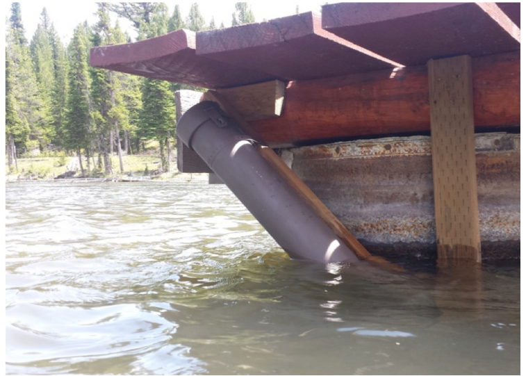
Figure 2 - An image of the Flat Rock sonde housing, which is affixed under the upstream end of the Flat Rock Club's dock.
